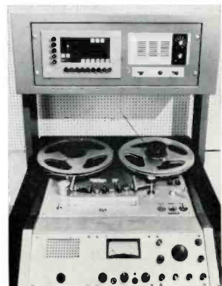
Figure 2. A reel-to-reel tape recorder with its selector module used at ABC radio.
